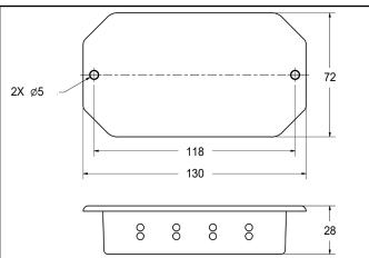
Figure 4. Mounting hole locations of the Control Unit (dimensions in mm)
