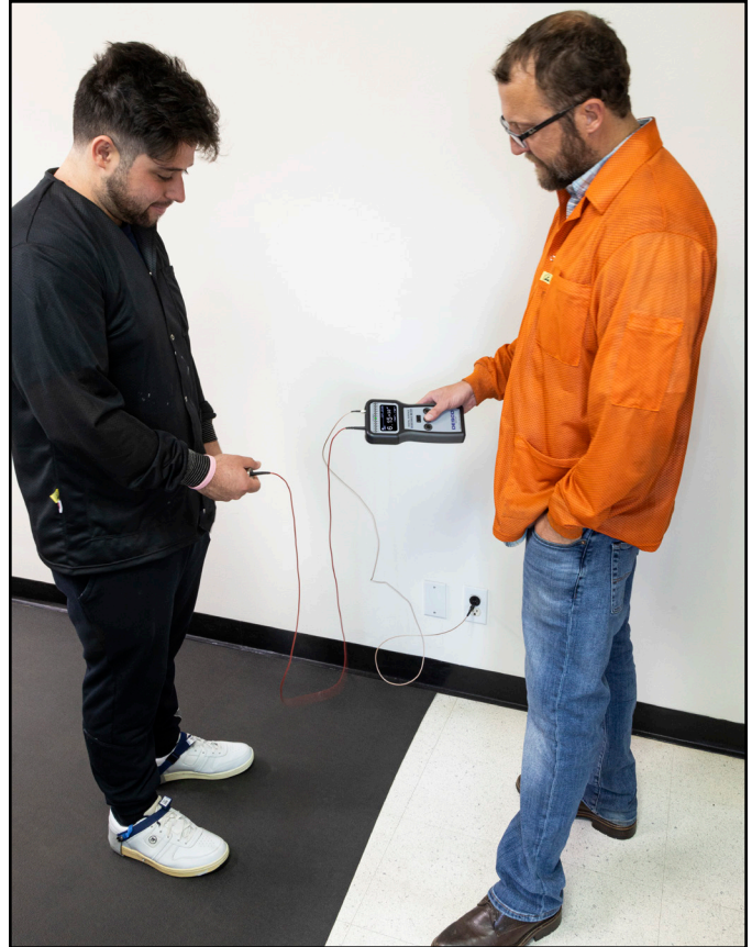
Figure 10. Using the Desco 19295 Handheld Electrode to measure Floor Materials and Footwear - Resistance Measurement in Combination with a Person (IEC 61340-4-5)
