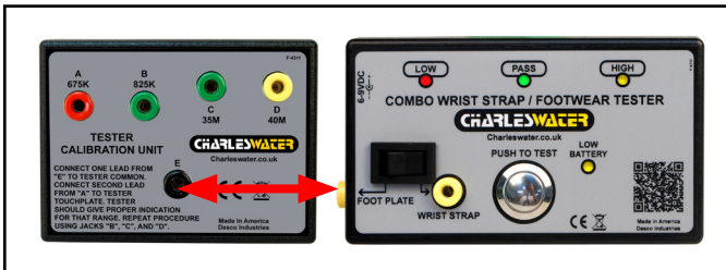
Figure 4. Connecting the test lead from banana jack “E” on the Calibration Unit to the FOOT PLATE banana jack on the Combo Tester
