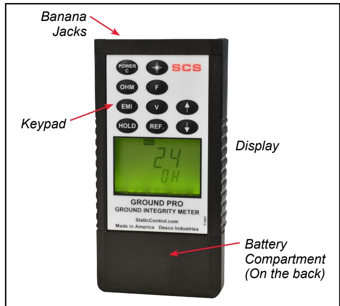
Figure 2. Ground Pro Meter features and components
