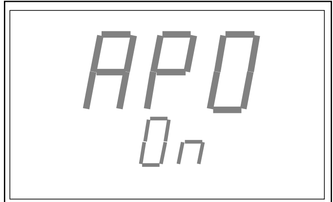
Figure 4. Automatic power on/off indicator.
